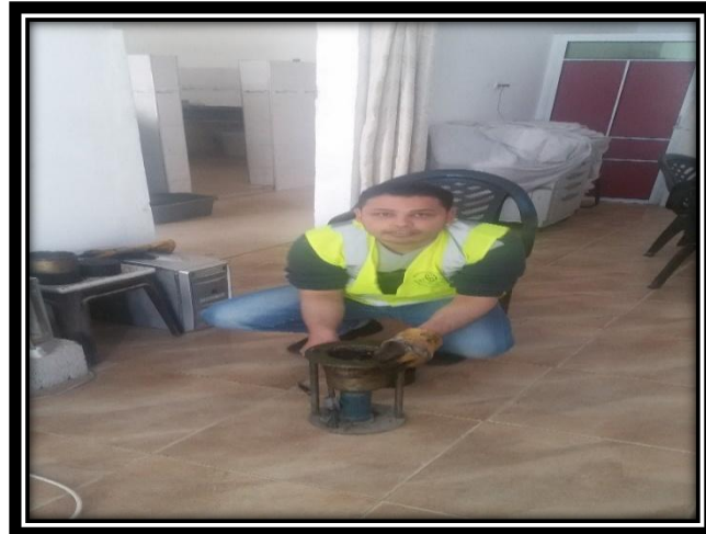
Figure E.4: Removing Marshal Samples after compaction
