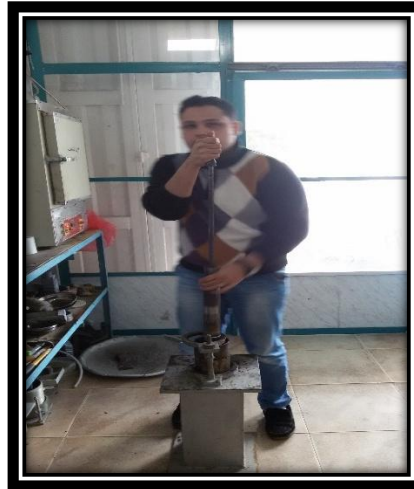
Figure E.10: Asphalt mix during compaction
