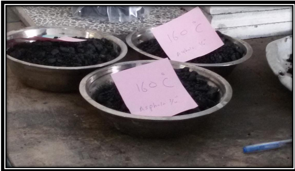
Figure 3.10: Preparation of asphalt mix at 160 C°
