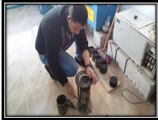
Figure E.6: Removing Marshal Samples after compaction
