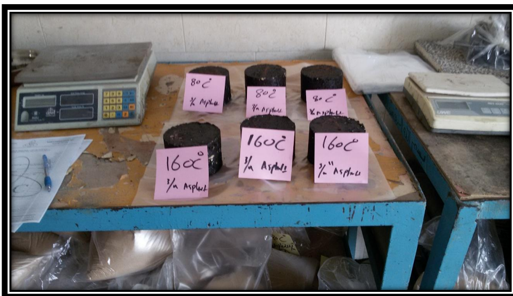
Figure 3.11: Asphalt compaction temperature at 80C° and 160C°
