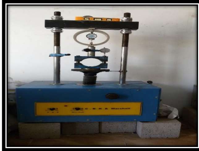
Figure E.9: Testing Marshall Samples for stability and flow
