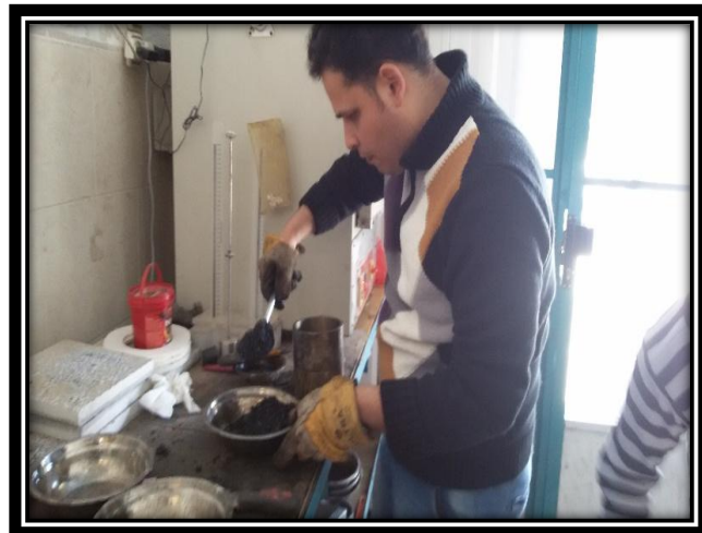
Figure E.5: Asphalt mix preparing in the mold
