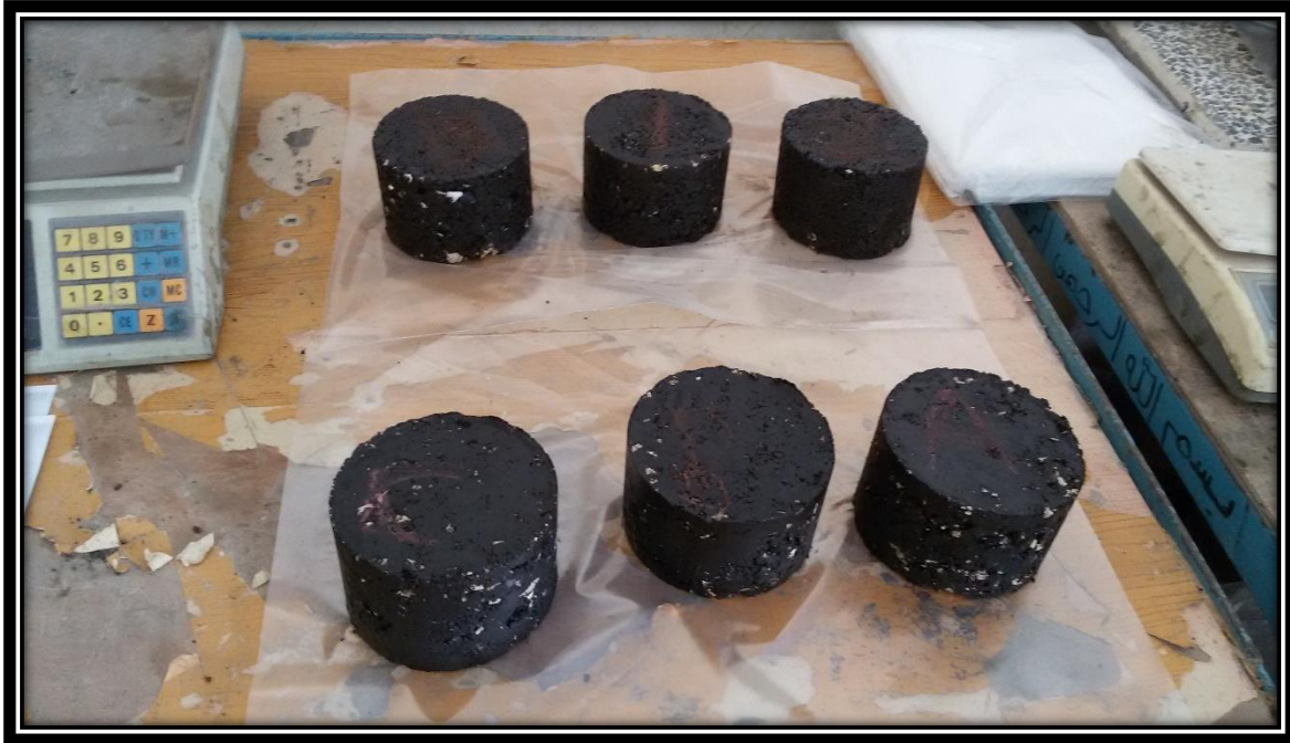
Figure 3.9: Marshal specimens for different bitumen percentages
