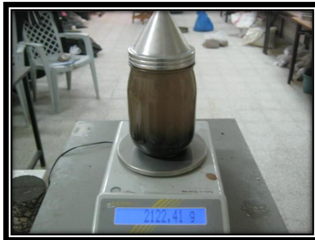
Figure E.11: Measuring the theoretical density using pycnometer
